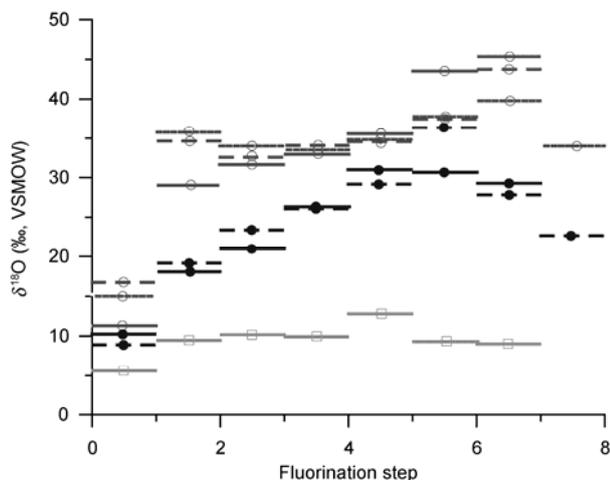
**Figure 2** Conditioned stepwise fluorination. Open circles represent modern diatom samples from Lake Sihailongwan, solid circles indicate diatomite, and squares represent NBS28.
