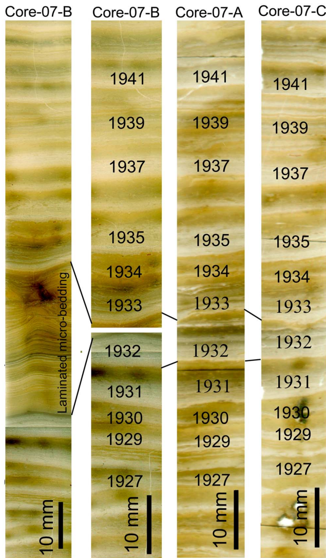
Figure 3. Scanner photos of thin sections showing a reworked layer. Microlaminated bedding, a reworked layer, is only observed in Core-07B (first column). In the second column, the microlaminated bedding was cut for comparing with other cores. The depths for AD 1941 in Core-07A, Core-07B, and Core-07C are 19.1, 18.6, and 20.2 cm, respectively. The depths for AD 1927 in Core-07A, Core-07B, and Core-07C are 25.8, 24.9, and 26.6 cm, respectively.
