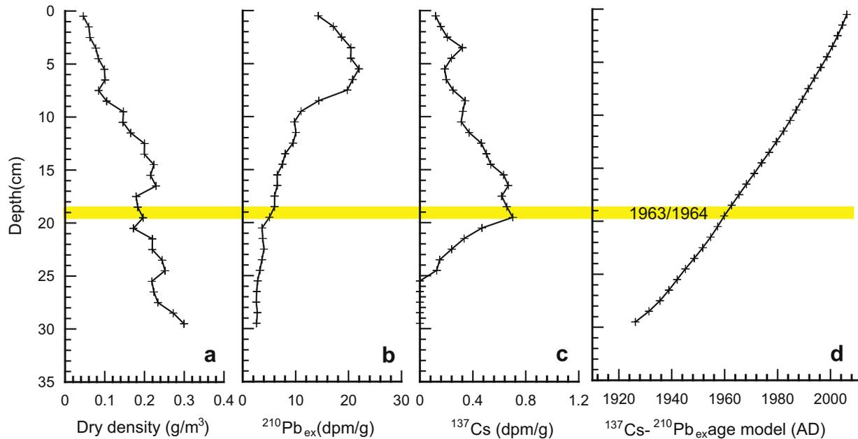
Fig. 3. HML short core  $^{137}\text{CS}$ – $^{210}\text{Pb}_{\text{ex}}$  age model diagram. a. Dry bulk density of sediment. b and c. Concentrations of  $^{210}\text{Pb}$  and  $^{137}\text{Cs}$ . d.  $^{210}\text{Pb}$  and  $^{137}\text{Cs}$  age model.
