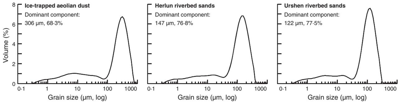
**Fig. 8.** Frequency distribution curves of modern aeolian dust trapped on the ice in the central part of Hulun Lake and modern riverbed sands deposited at the mouths of the Herlun and Urshen River. The modal size and percentage of the dominant component of each sample are shown.
