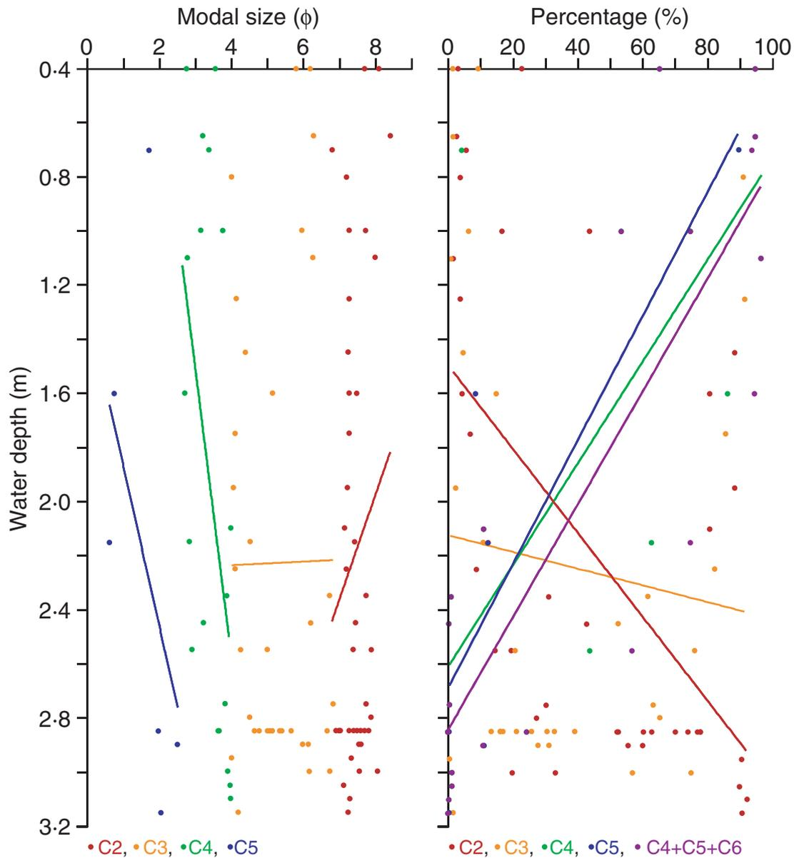
**Fig. 6.** Modal size and percentage of the grain-size components in 40 samples from the surface sediments of Hulun Lake plotted against water depth. Linear regression lines are shown. For the regression equation, correlation coefficient and standard error, see Table 3.
