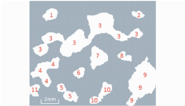
图5 连通区域标记结果示意图 Fig. 5 Tagging results of the connected regions
