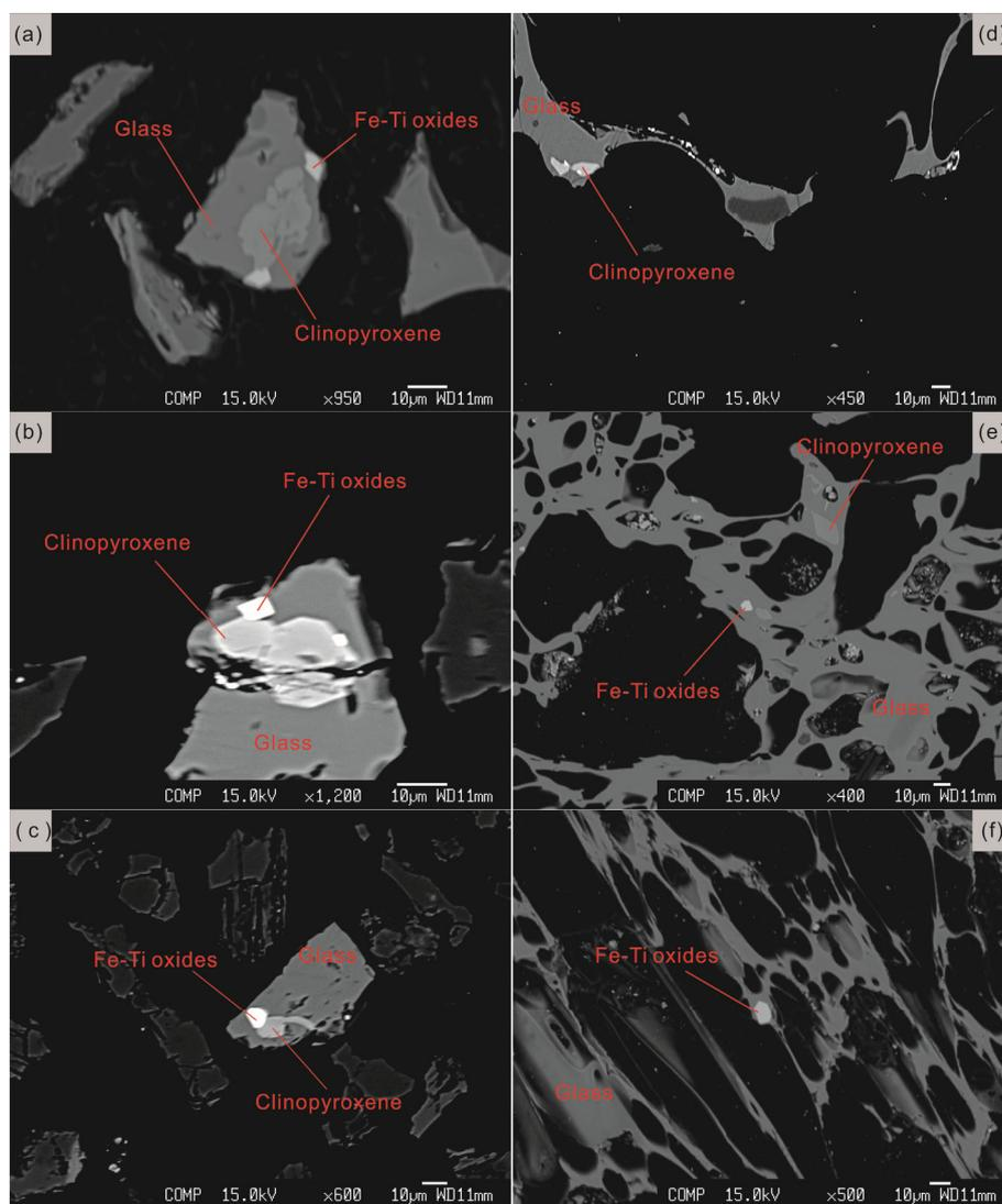
**Figure 2** BSE images for the distal tephra from Lake Sihailongwan ((a)–(c)), proximal dark pumice from Changbaishan ((d), (e)), and proximal light pumice from Changbaishan (f). The scale bar is 10 μm.
